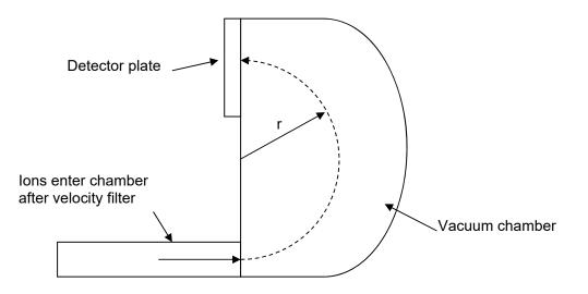
a) Indicate on the diagram the direction of the magnetic field in the vacuum chamber required to produce the semi-circular path shown.
